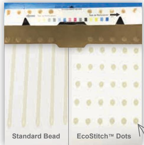
*EcoStitch™ dot pattern maintains bond integrity and achieves strong fiber tear, all while using less adhesive*
